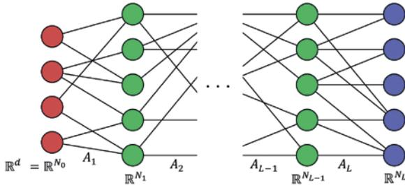
Fig. 1: Visualization of an artificial neural network as a graph. The nodes correspond to the neurons ( $N_l$ -many in the  $l$ -th layer), while the edges indicate which neurons are connected between the different layers (specified by the weight matrices  $A_l$ ).
